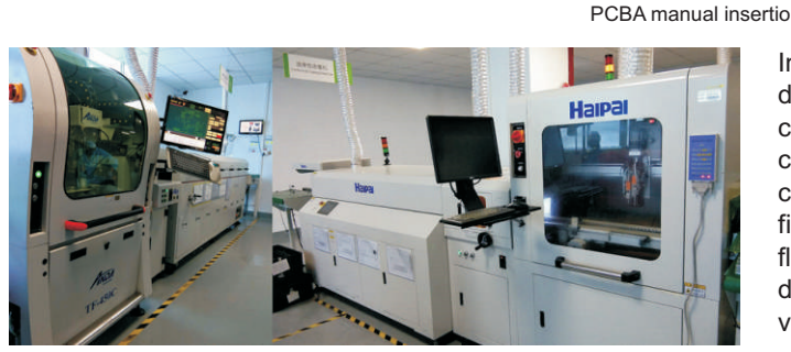
SMT automatic paste produce line
